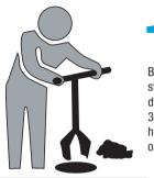
Begin by boring a starter hole 3" to 5" in diameter and 18" to 30" deep. Bore this hole with a hole digger or hand auger.
