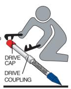
To drive the point use either a sledge hammer or a 2" or 3" pipe with a weighted end, also called a steel post driver.
